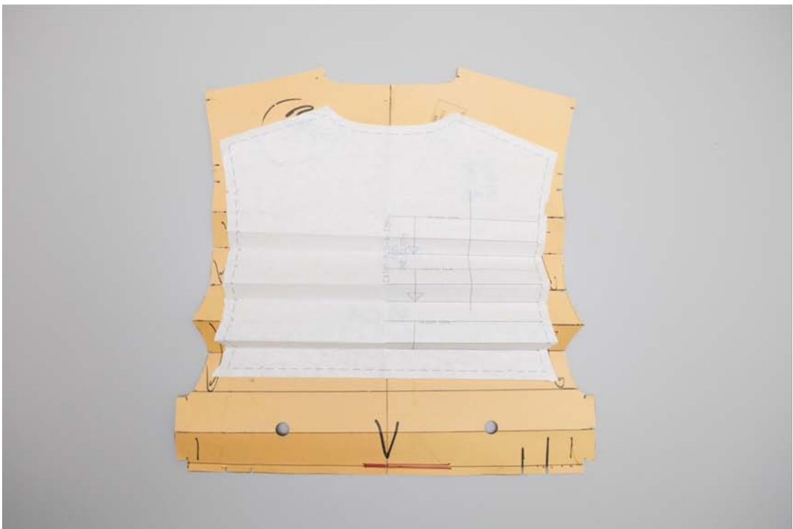
Pattern pieces A and B showing the difference of body fit and pleat size.
